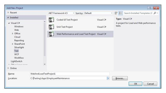
The above option will create the new project, add the web performance test to the project, and then open the recorder as well.
