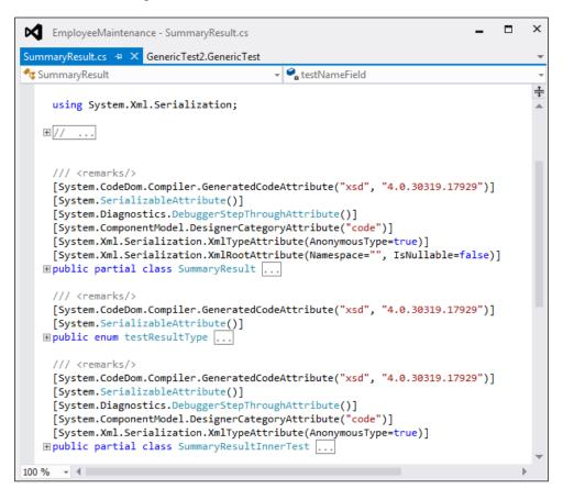
There are two classes as SummaryResult and SummaryResultInnerTest each contain the same methods. SummaryResult collects the overall summary of the Test Run and SummaryResultInnerTest collects the details of the individual tests within the application under test. The following screenshot shows multiple methods within the SummaryResultInnerTest class:
