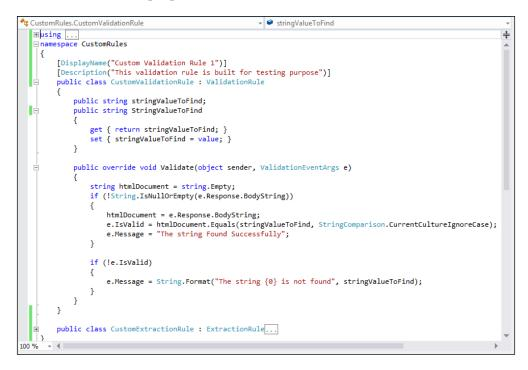
The Validate method contains two parameters: object and ValidationEventArgs. The ValidationEventArgs object contains the response property that provides the response text for the request through which the string value can be found and the response validated.
