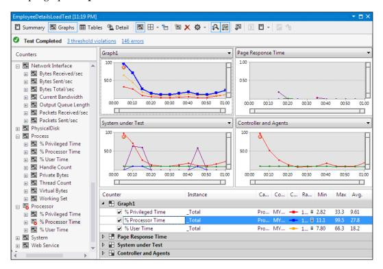
The **Graph1** is the new graph added to the result with a few processor related counters added to it. The counters and readings are listed in the table below the graphs.
