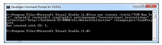
The Test Run is created and the result can be viewed in **Test Manager** for analysis. Open the **Test Manager** and select the option **Test** under **Testing Center**. Select **Analyze Test Runs** from the menu bar. The **Analyze Test Runs** window shows the Test Runs for the Test Plan. The following screenshot shows a detailed view of the Test Run. The test is still in progress but you can see the test cases and the other details provided at the command:
