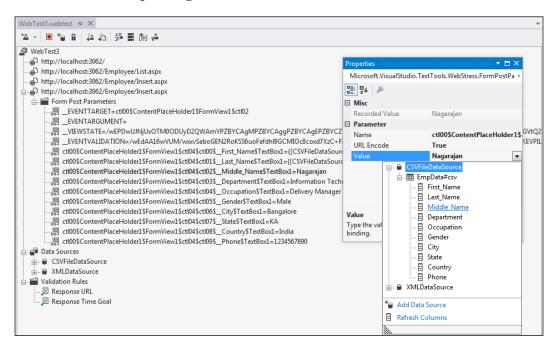
You can see the value assigned to the **Form POST** parameter. The first name parameter is bound to the **First\_Name** field in the selected data source as follows: {{CSVFileDataSource.EmpData#csv.First Name}}
