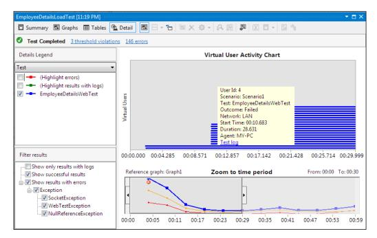
Pointing to any of the line in the activity chart shows a tool tip message for the selected user with all the activity details like virtual user ID, scenario, test name, test outcome, network, start time of the test, duration for the test, and the agent on which the test was run.
