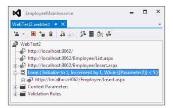
8. Now everything is set for the looping of the same request with the incremental value of **Parameter2**. Select the web performance test and run it. The Test Runs with the **Parameter2** value getting incremented every time the test is run. The test stops when the context **Parameter2** value becomes 5. The following image shows the end result of having four new users or employees added to the stem:
