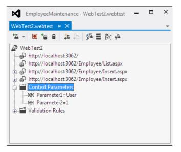
3. Open the **web test** folder and expand the request that captures the insert operation. The web performance test captures all the details under the **Form Post Parameters** for the web request. Let's use the same details for multiple user or employee creation, except the **First Name** and **Last Name** which will differentiate the users or employees.
