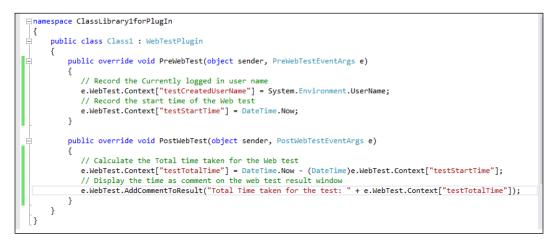
Add this project reference to the **Web Test** project. Then select the **Web Test** project and choose the **Add Web Test Plugins** option from the toolbar which lists the classes within the assembly. On selection of the class, the class for the plugin gets added to the Test Project:
