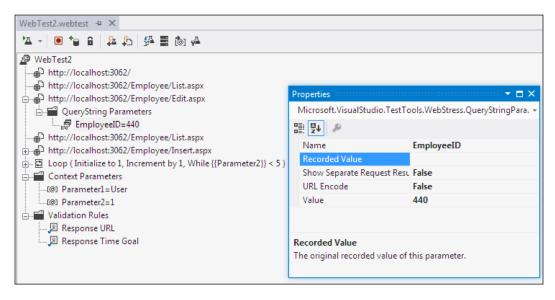
Setting properties values and usage of the QueryString parameters are same as the **Form POST Parameters** properties, except the additional property which is **Show Separate Request Result**. This is used for grouping the requests based on the value of this query string parameter. This is very useful for load testing for grouping a bunch of requests based on this field value. The default is False.
