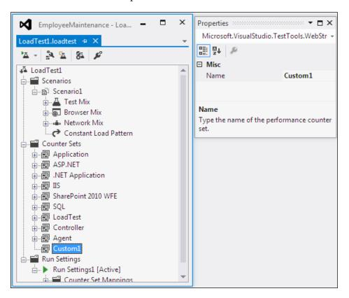
Now select the counter, right-click on it and choose the **Add Counters** option and select the category, and pick the counters required for the custom counter set. For example, add counters to collect the **Network Interface** information, such as number of bytes sent and received per second and the current bandwidth during the test. Select these counters for the counter set.
