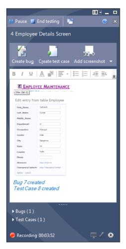
If the exploratory testing is complete, click on the **End Testing** option at the top of the recording window. This option closes the recorder and opens the **Testing Center** showing the details of the completed session. The summary shows the start and completed date time, test settings used for the test, build associated to the testing, the owner, and the work item with which this exploratory testing is associated.
