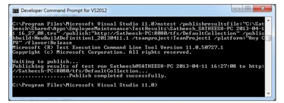
The command line options used in the preceding screenshot shows the Test Result trace file, TFS Team Project, and build against which the Test Result should be published. The command line also has the platform and the flavor values matching the build configurations.
