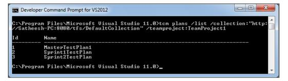
To list all the Test Suites within the Plan, use the following TCM command with the options as shown in the next screenshot along with the Plan ID, collection, and the Team Project name. Use the Plan ID from the previous command output:
