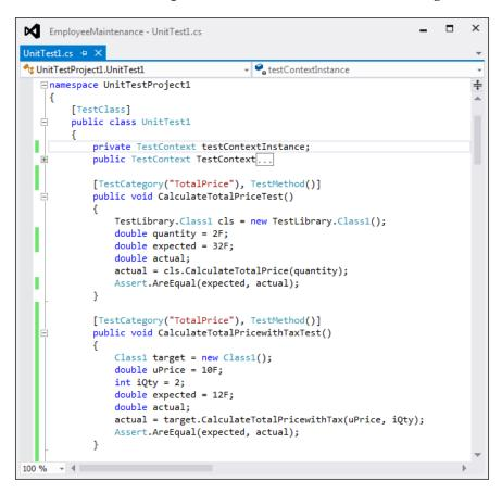
For any tests created using Visual Studio, the TCM utility can be used to import it to the Test Plan in **Test Manager** as test cases. The following command imports all tests with the category defined as TotalPrice from the **UnitTestProject1** assembly into the Team Project **TeamProject1**. The category is defined to the tests to group it from all other available tests within the assembly. Refer to the following screenshot:
