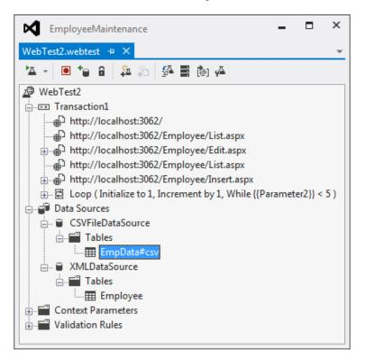
Once the data source is added, change the source of the **Form POST** or **QueryString** parameter values. To do this, select the **Form Post Parameter** under the web request, then right-click and choose **Properties**. In the **Value** property, select the data source and select the corresponding field from the data source as follows:
