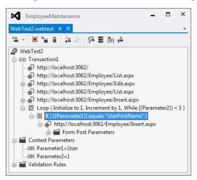
The web test request will not get executed because of the failure of the condition as the parameter is not the same as expected. The following result shows the execution of the condition and action based on the condition result:
