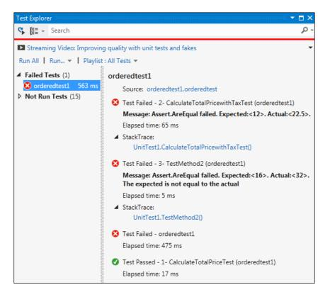
The **Test Explorer** window also provides detailed information about the tests run. Select a test that is being run in the explorer to see it. This information includes the link to the source code where the test fails, followed by test name and the message from the test method for failure, the elapsed time for the test, and stack trace for the test. The total duration of the ordered test is also shown next to the ordered test failure status under the failed tests section.
