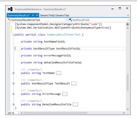
The third-party tool can make use of this class file to write the Test Result details, or the test application should take care of writing the Test Result details into the XML file based on the XML schema used. The results output XML file should look like this:
