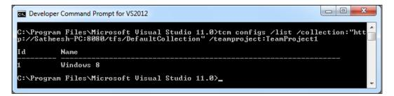
The following is the command and output for listing all the Test Plans within the Team Project:
