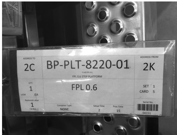
Figure 5.3 Example of a Kanban card used to trigger replenishment of finished goods.
