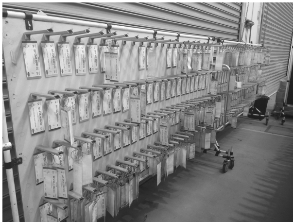
Figure 7.1 Example of a Kanban control board. As materials are consumed, Kanban cards are returned to purchasing, triggering ordering. The cards then stay on this board until the materials are delivered, and then the card is removed and attached to the new material containers.
