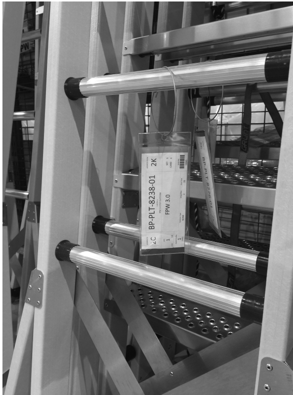
Figure 5.4 Kanban cards attached to finished ladders.
