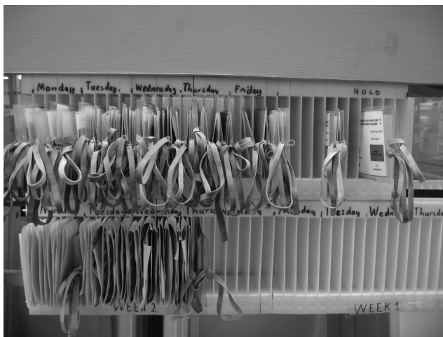
Figure 5.5 Load leveling box. When the ladder in Figure 5.4 is sold, the Kanban card is detached and returned to this box to trigger replenishment.
