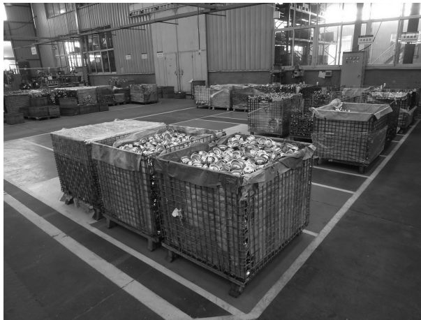
Figure 5.6 Example of color-coded Kanban squares. When the bins are emptied and the yellow area on the floor exposed, this triggers replenishment. Exposure of a red area highlights potential shortages and triggers expedited replenishment.
