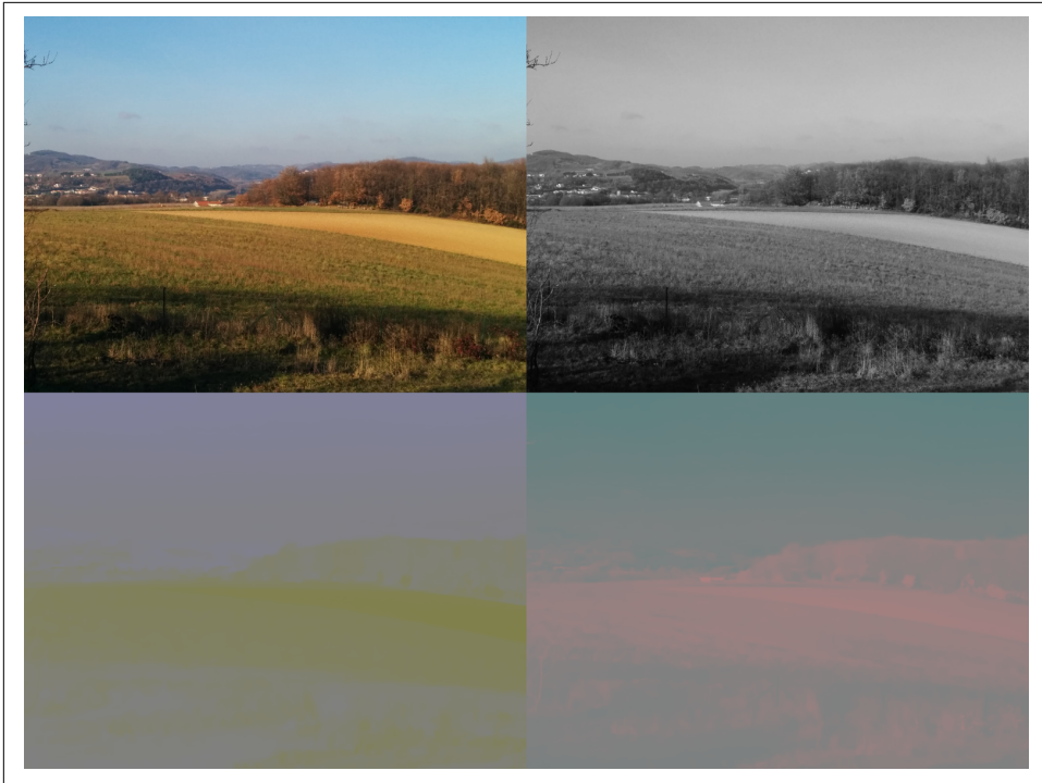
Figure 2-6. French countryside in winter, top to bottom, left to right: full image, Y component, Cb component, and Cr component
