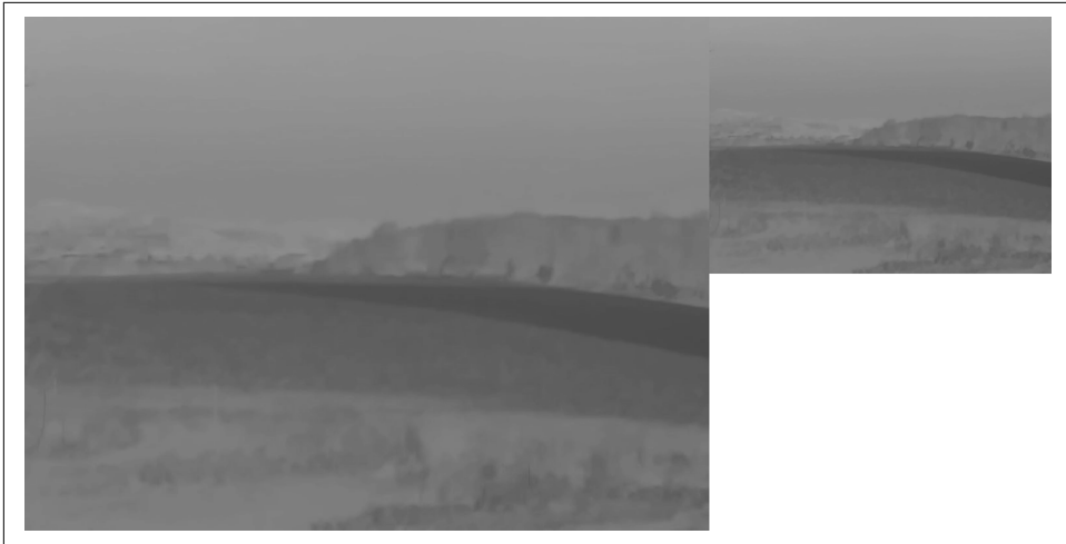
Figure 4-4. To the left, the original (untainted) Cb component; to the right, the same component after 4:2:0 subsampling
