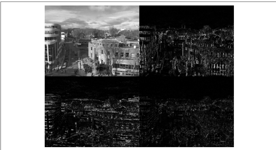
Figure 5-2. Image after Discrete Wavelet Transform (details enhanced for demonstration purposes)
