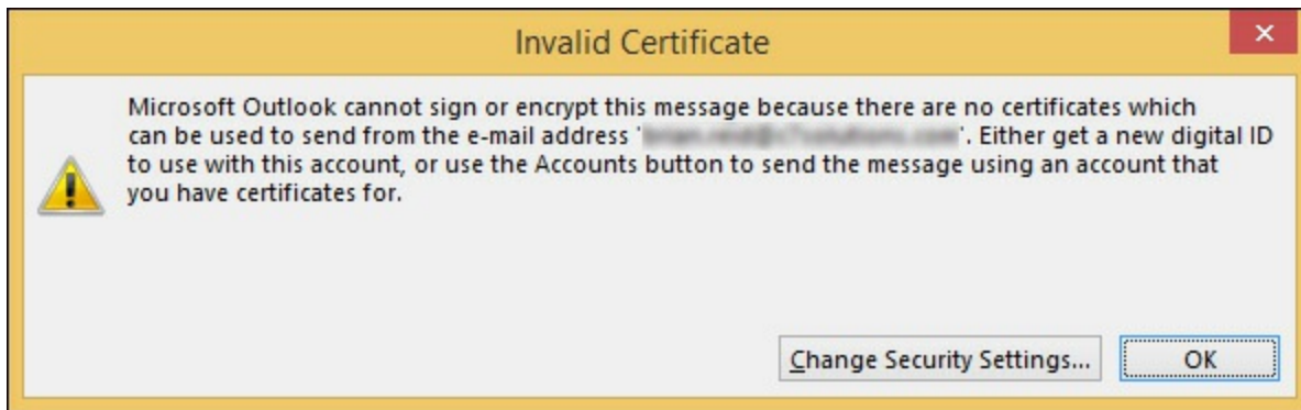
FIGURE 3-12 The Invalid Certificate error when you do not have your own encryption certificate
