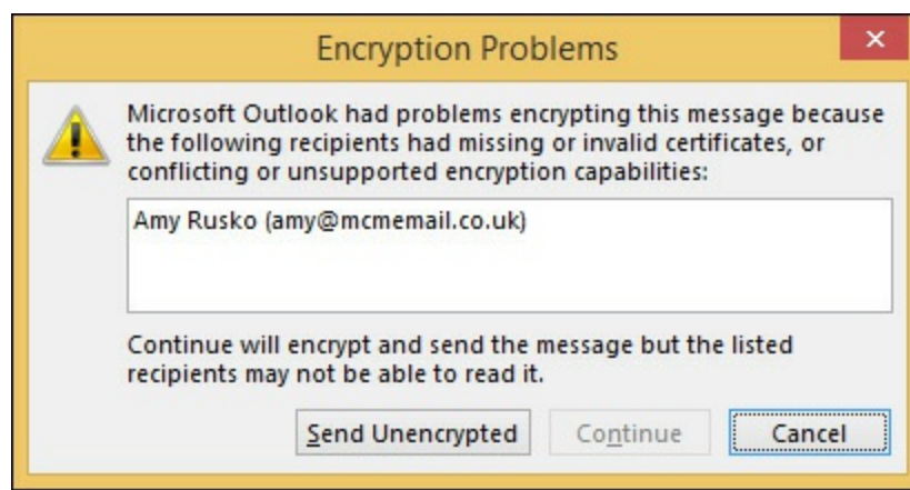
FIGURE 3-11 Encryption Problems dialog box when sending to users whose public key you do not have
