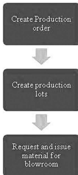
Figure 4.3 Pre-production flow in spinning ERP
