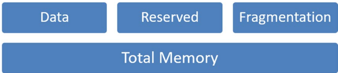
Figure 3-20. This is how the total memory of a Redis instance is allocated. Despite the graphic does not suggest proportions, we should consider we have not the total amount of memory available for data
