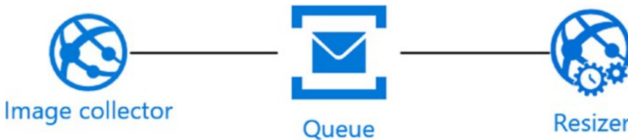
Figure 6-1. The simplest scenario where a producer enqueues images for further resizing in a different component
