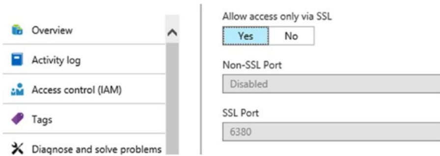
Figure 3-28. This let us disable the non-SSL port, which may permit man in the middles to read the traffic from/to the cache
