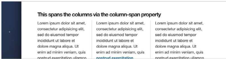
FIG 7.6: Use column-span to make an element defy the columns and span the full width.
